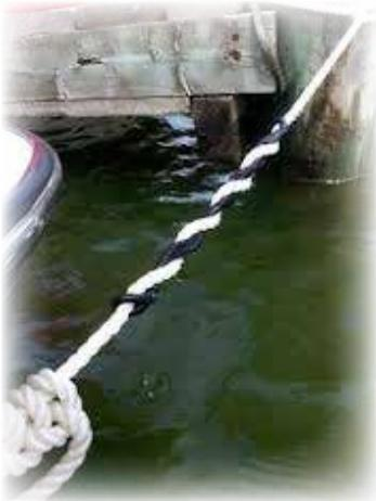
A snubber will take the jerking strain off the line. Many boaters use a device such as this at all times
