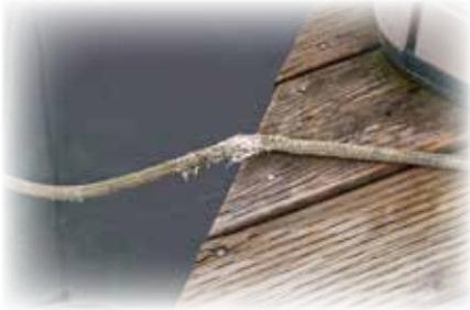
Chafing will wear out a good line quickly in rough conditions. Anti-chafing devices protect the line’s condition effectively.
