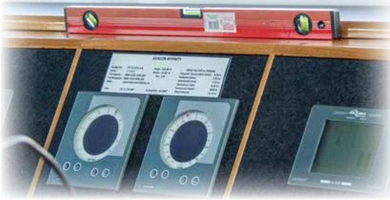
The river boat, 300 feet long has a high tech instrument for displaying the degree to which the boat lists. It's called a carpenter's level. Honestly!
